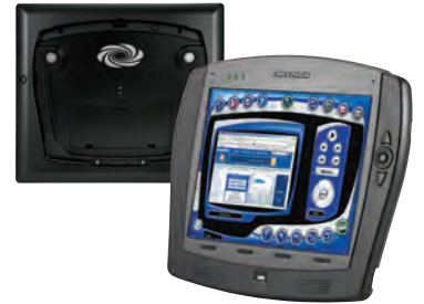
8.5" WiFi 802.11a/b/g Touchpanel with embedded PC applications for Web browsing, streaming media and email, and built-in audio and video. Optional desktop docking station available.
